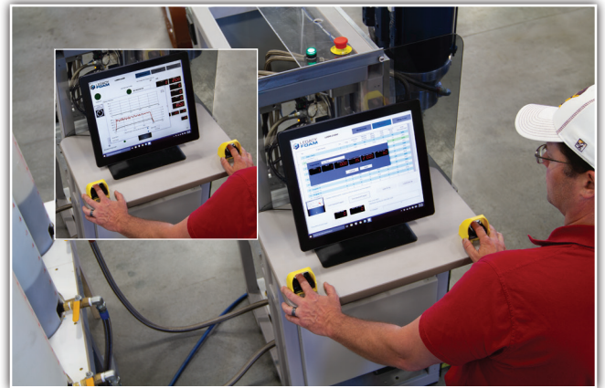
Computer controlled PLC with finger switches for operational safety.
