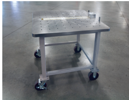
Portable heavy-duty steel molding table with bottom fill design. Threaded table-top allows operator to clamp down various sizes of molds quickly and securely.
